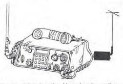
range and is very vulnerable to jamming. Nomad packs use these to communicate with other packs, so they are not as vital as internal communications gear is. This unit weighs about ten kilos and requires considerable power. No one really makes these anymore, and even the nomads are upgrading to better gear.
